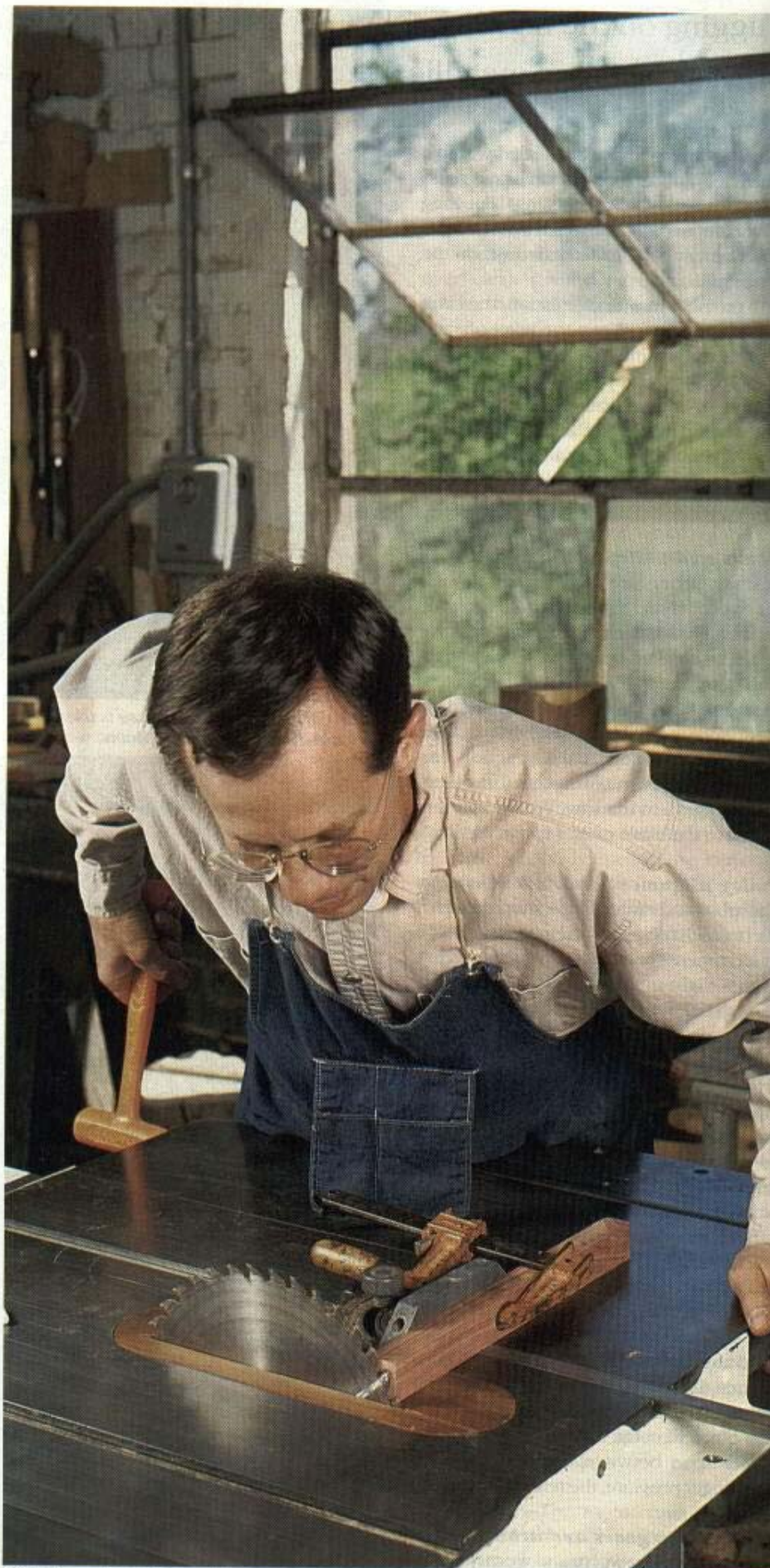
Tap the edge of the table to nudge the miter-gauge slot parallel to the blade.
