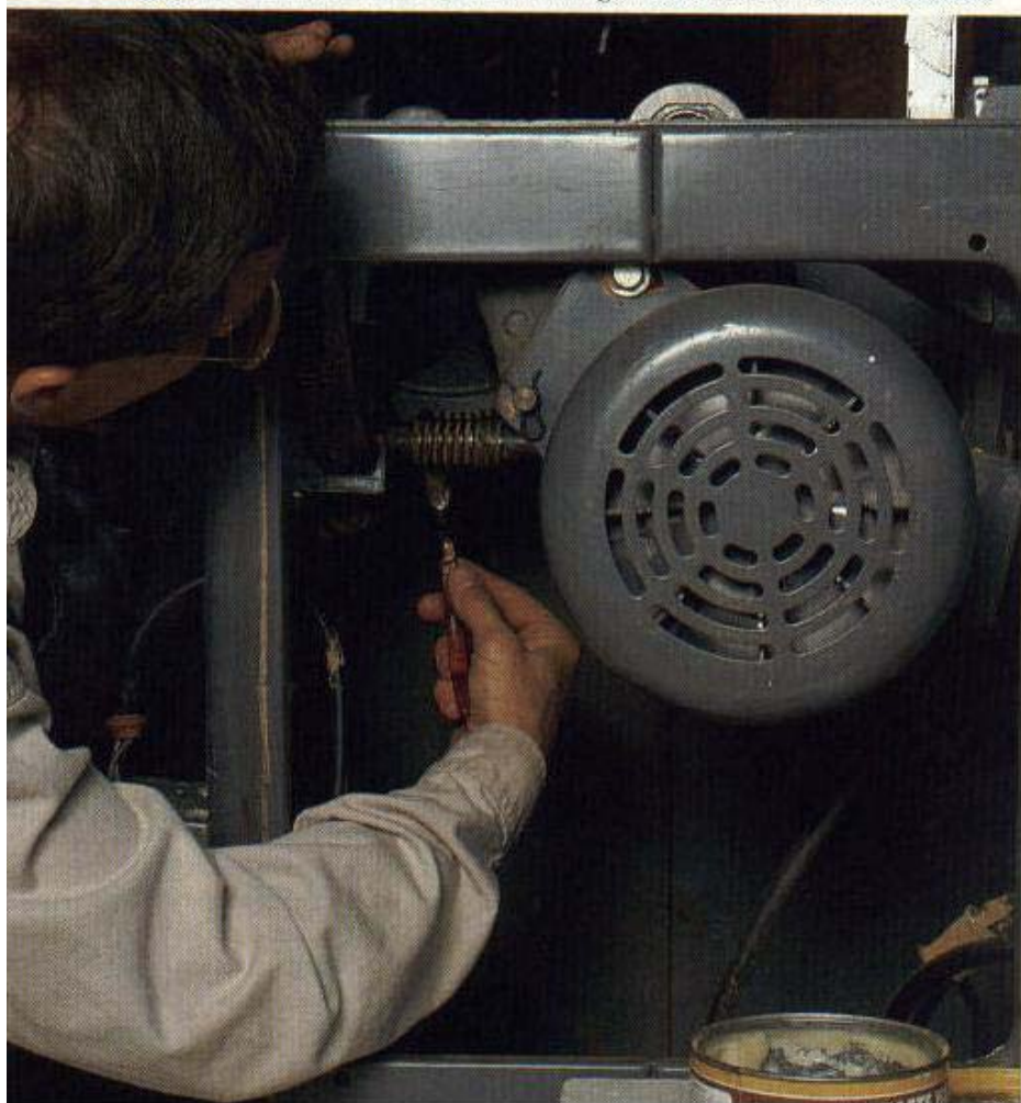
Paste wax applied with a toothbrush lubricates gears and doesn't attract sawdust.
