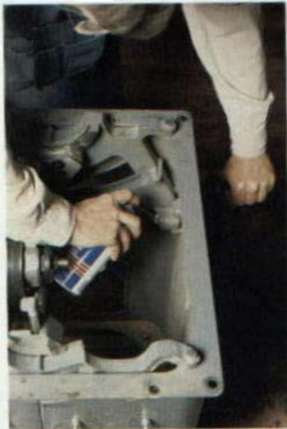
White lithium spray grease is used to lubricate the hard-to-reach pivots.
