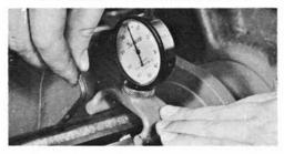
Proper use of Micrometer Knife setting gauge will maintain equal knife height, assuring a smooth, even planed surface. Check knife height with Dial Indicator immediately upon receipt of your new machine. Knives are set approximately  $\frac{1}{16}$ " above high point of chipbreaker in knife locking shim. When knives are ground or a new set installed, care should be taken to re-set to original height.
