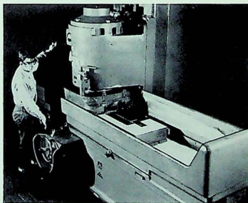
18" x 18" x 60" HILL "Openside" Vertical Spindle Grinder with 18" x 60" magnetic chuck grinding steel shim plates in a large west coast steel mill.
