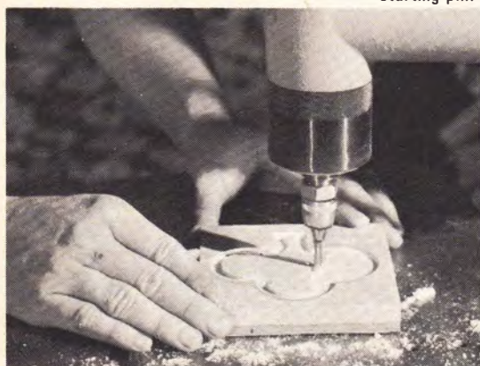
Routing using a guide pin and template.
