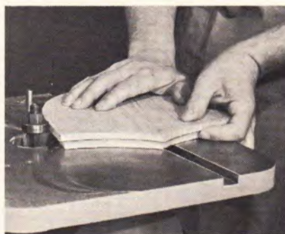
Free-hand shaping irregular stock using a starting pin.
