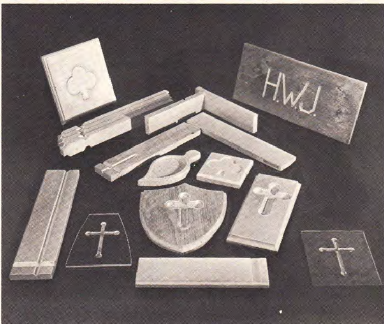
Shown are typical operations that may be performed on wood, plastic and aluminum on the Rockwell Delta Overarm Router/Shaper.
