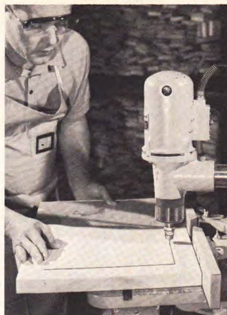
Placing a decorative bead on a door panel.
