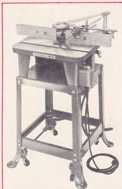
Wood Shaper (Bench Model) with Accessory Ring Guard and Spring Hold Downs.
