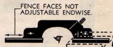
ON MOST SMALL SHAPERS ONLY THE FRONT HALF OF THE FENCE IS ADJUSTABLE.
