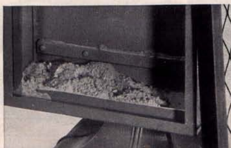
Right, rear view of dust-collecting unit on grinder, showing the dust filter. Note the very large area of the filtering surface. This large area lowers the velocity of the air passing through it and permits the filter elements to collect the maximum amount of the fine, invisible dust particles.
