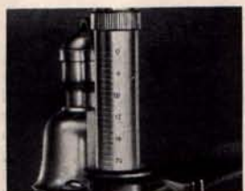
Tension of spring can be adjusted to suit blade, and graduations on tube and adjustment.
