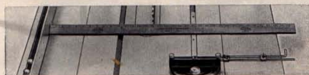
Photo above shows the great capacity on the right of the blade, enabling the user to rip to the center of 48" stock. The photo at left shows how the rip gage can be used up to 15" from the left side of the blades—a feature of great value in many operations.
