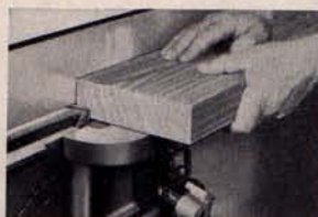
Left: Rabbets a full \frac{1}{2} " deep can be cut at one pass. The guard is instantly removed for rabbeting, and just as quickly replaced.
