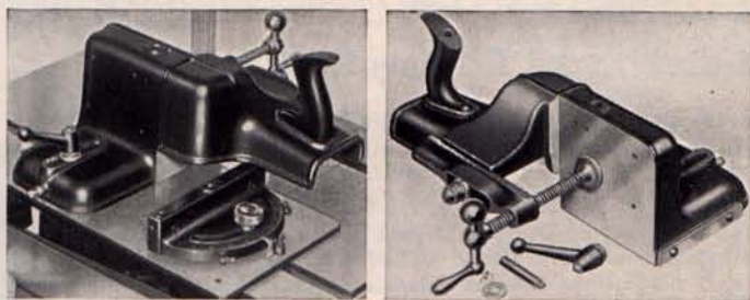
At left, rear view of tenoner mounted on base plate of No. 1186 sliding jig. No. 1172 is similar, but the miter-gage head is not furnished. View at right shows No. 1170 tenoner as furnished without base plate, for use in connection with No. 1186 jig.
