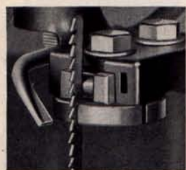
Highly efficient disk blade guide and roller support.
