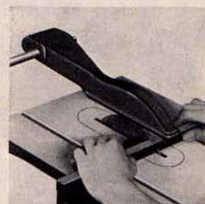
Cutting a steel bar with the abrasive wheel, showing No. 230 Guard.
