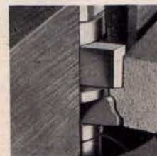
Making a combination rabbit and ogee cut on sash stock, using a spacing collar between cutters.
