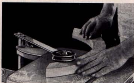
Shaping a curved rail with the No. 982 guard in place. Note how completely the knives are covered.
