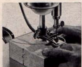
Work up to 2" thick may be cut on this saw.
