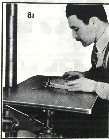
The drill press will make an emergency shaper producing good results provided that the cutting is not too heavy. The drill press head may be used for shaping operations either in the regular or inverted positions as shown in Figs. 80-83.
