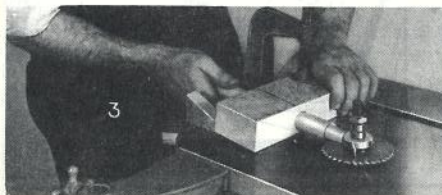
Fig. 3 shows tenoning of round stock.
