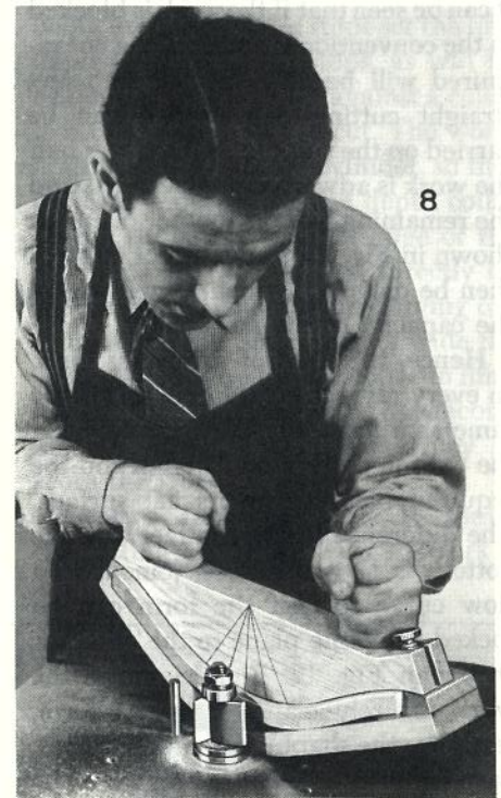
Edge shaping a chair-back rail with the use of a rocking form is shown in Fig. 8.
