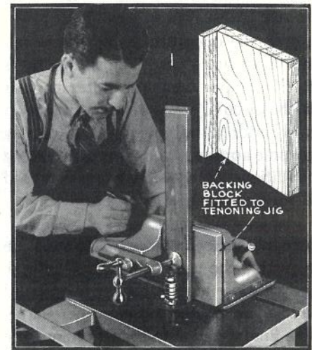
Fig. 1 shows how the circular saw tenoning jig can be used to good advantage for many shaper operations.
