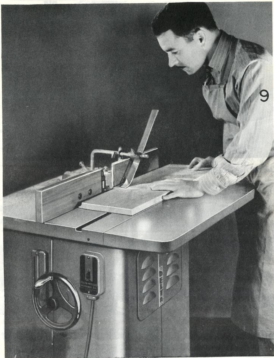
THE SHAPER . . . Top ranking production tool for the small shop and capable of a score of different operations, some of which are impossible in any manner. Photo above illustrates cabinet model with \frac{3}{8} inch spindle. The machine should be located in an unobstructed working space.
