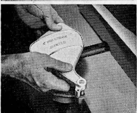
Knife guard completely covers knives and slides back out of the way with the work. Instantly removed for rabbeting and as quickly replaced.
