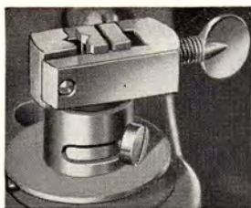
Lower chuck of steel. Light but strong and holding all blades.
