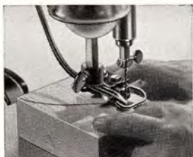
Work up to 1 1/4" thick may be cut on this saw.
