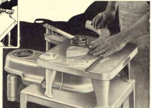
The Circular Guard Should Be Used Whenever Possible When Shaping Directly Against Guide Collars.
