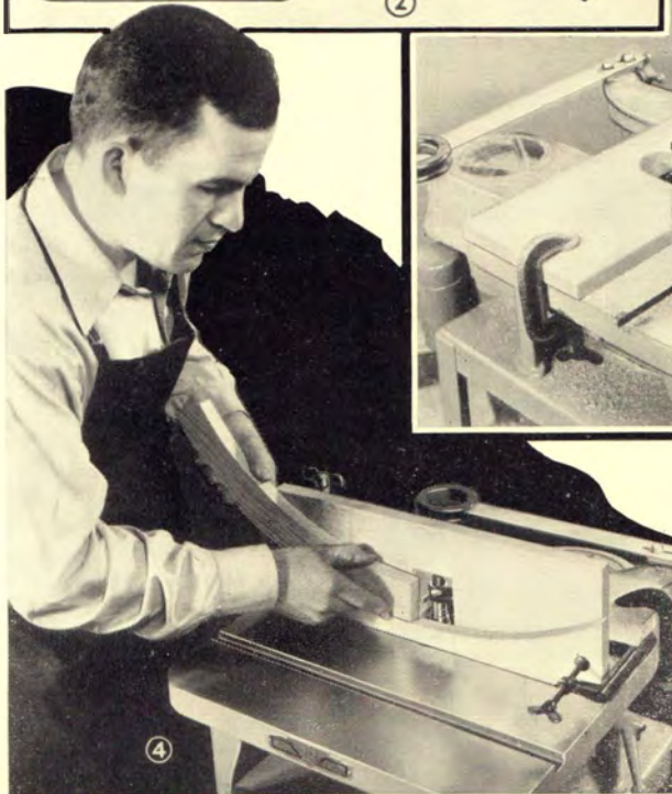
Construction and Manner of Using Segment Guides for Curved and Circular Work.
