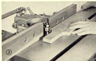
Above, Taper Jointing on the Shaper. At Left, Making a Heavy Cut.
