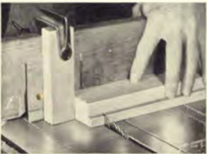
To secure the required 1/4 inch offset, the shoulder on the long side of the tenon is cut on the circular saw, 1/2 inch from the end and level with rabbet.
