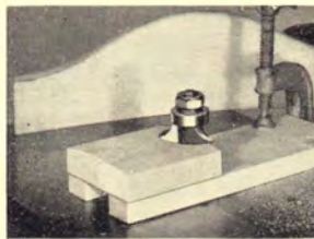
A wood guide block is necessary when shaping compound curves.
