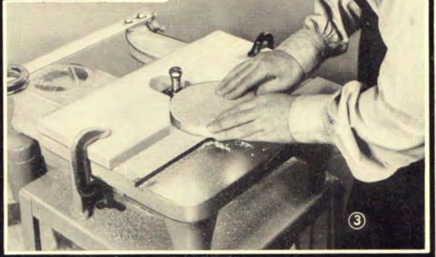
Construction and Manner of Using Segment Guides for Curved and Circular Work.
