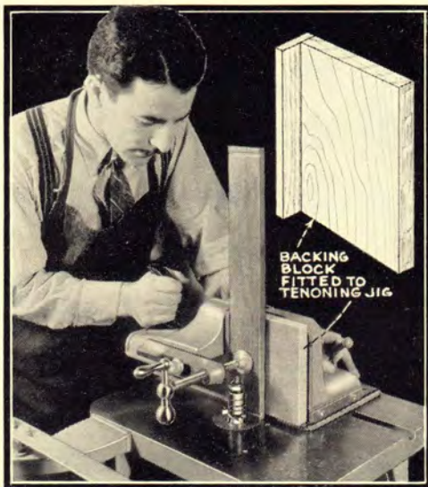
The Circular Saw Tenoning Jig can be Used to Good Advantage for Many Shaper Operations.
