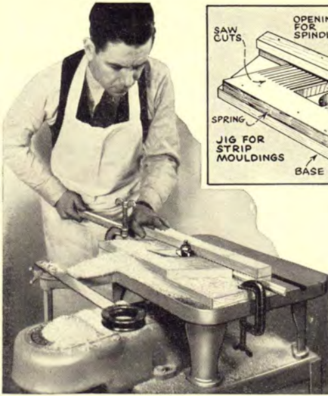
Strip Jig Above and Photo to Right Show How Hold-downs Are Used in Shaper Work.
