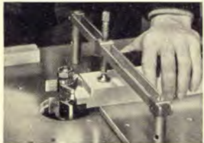
The two stock sizes of Delta straight shaper cutters combine with the saw cut to produce the 1/4 inch offset tenon.
