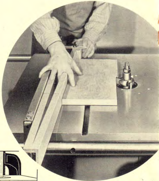
Above, using tapering jig in connection with rip fence. Left, two methods of cutting tenons.
