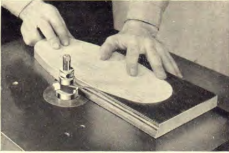
Above, using a sliding starting block. Right, path of shaper cutter.
