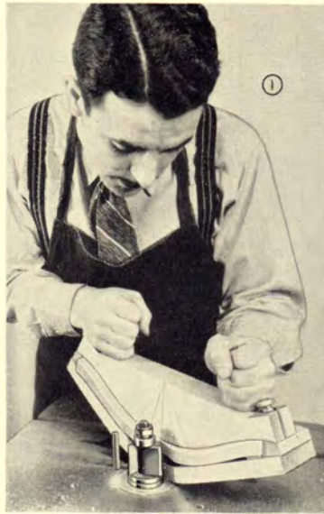
Edge Shaping a Chair-Back Rail With the Use of a Rocking Form.
