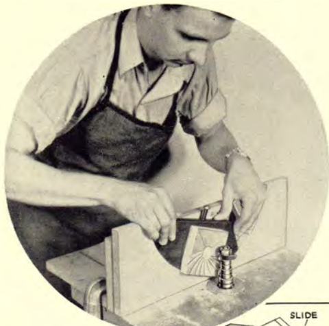
Ornamental Radial Rosettes in a Wide Variety of Patterns Can Be Made With the Simple Jig Shown.
