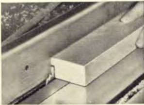
The glass rabbet can be cut in a number of different ways. As good a method as any is the "two pass" cut with a single saw blade, as shown.
