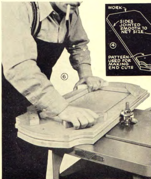
Above, Using a Built-up Outline Pattern for Shaping the Edge of a Small Table Top.
