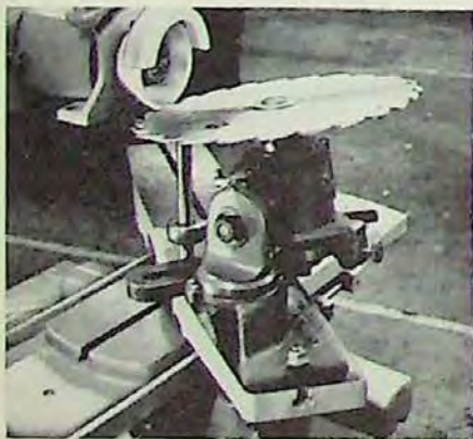
Sharpening a 16" carbide-tipped saw blade using the 24-955 Unihead.
