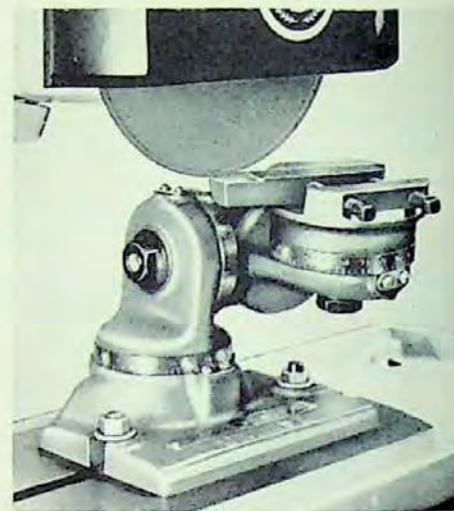
Using a diamond wheel to grind the chip-breaker groove on a tool bit using the 24-902 Univise.
