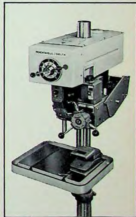
Shown is the Automation and Remote Control Kit with foot switch mounted on a Delta Power Feed Drill Press.
