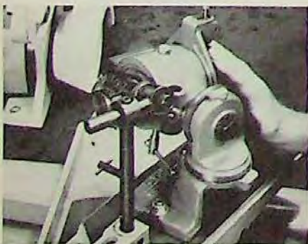
Grinding an angular cutter using the 24-955 Unihead.
