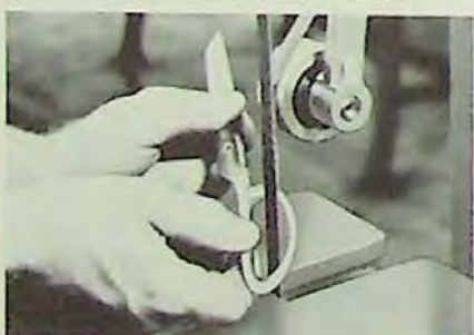
Scissors Manufacturer . . . using narrow belt, and without platen, internal grinds rounded edges with ease.
