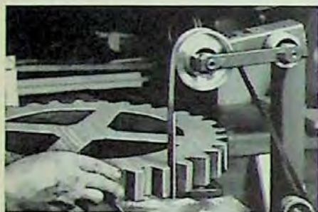
Pattern Shop . . . narrow band gets into small openings . . . finishes patterns rapidly to close tolerances.
