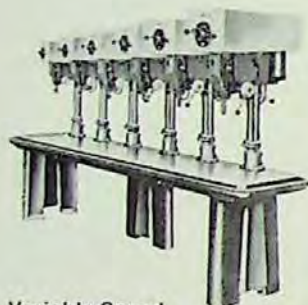
Variable Speed Multiple Spindle Model —Available in 2, 3, 4, 5 or 6 spindles with \frac{1}{2} " key chuck or No. 2 M.T. spindle, hand or power feed, on both Step Pulley and Variable Speed Models. Can be ordered as cataloged, or custom assembled (either at the factory or in your shop) using any combination of Step Pulley or Variable Speed Heads with any number of spindles from one to a drill press a block long if desired.
