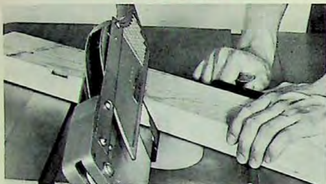
Big Capacity 9" Tilting Arbor Saw cuts stock 2\frac{3}{4} " thick; full 2" at 45° blade tilt . . . rips to the center of a 4-foot panel.
