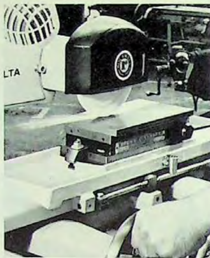
Grinding a precision surface on flat stock (magnetic chuck not sold by Rockwell).
