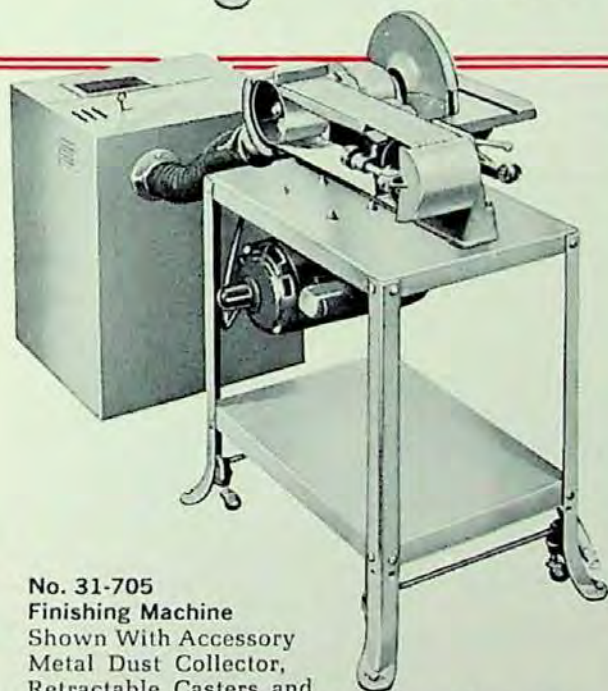
No. 31-705 Finishing Machine Shown With Accessory Retractable Casters and Electricals.
