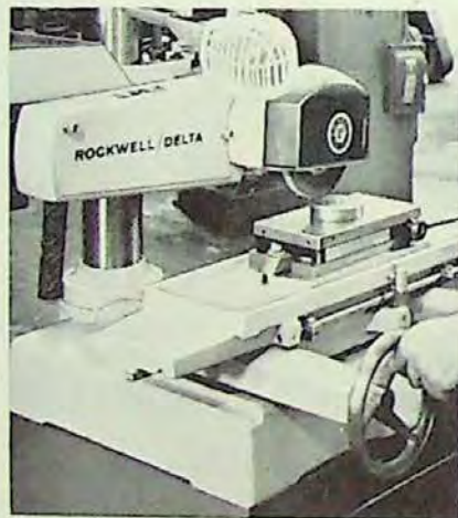
Applying a perfectly true, smooth finish to a part (magnetic chuck not supplied by Rockwell).
