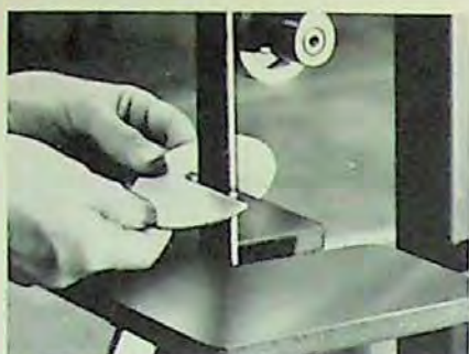
Assembly Department . . . quickly removes sharp edges on metal stampings, even in small openings.
