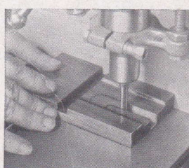
Routing against a guide fence, using the No. 974 spindle with \frac{1}{2} -inch hole.
