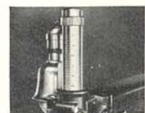
Tension spring over saw blade can be adjusted to suit the type of cut or the type of blade used.
