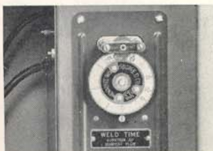
A NEMA Type 1AX timer provides for the so necessary weld time control. Range from 3 to 120 weld cycles. This normally expensive equipment is standard in the Delta Automatic Welder.
