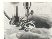
Big capacity for all jobs. Cuts up to 1 3/4" thick and the distance to the overarm is 24".
