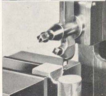
Set-up for a part placed in vise ready for machining.
