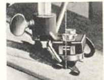
Spring hold-down functions even when table is tilted—giving added accuracy and ease of operation.
