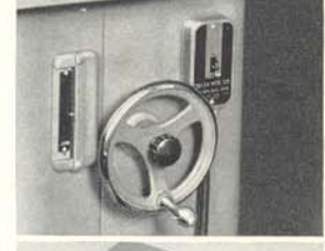
All controls in one group. Hand wheel for spindle adjustment . . . lock knob . . . scale showing spindle height . . . and starting switch.
