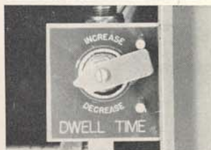
Automatic welding requires an off time control or dwell, before the horns reclose. This allows for proper weld spacing in stitch welding. Control is pneumatic and is simple to adjust.
