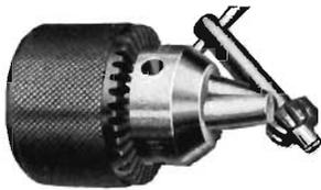
This Chuck is practical for general drilling work in the lathe. The jaws are of tempered steel and are operated by a heavy screw. The geared sleeve and key assure a powerful grip. Price and weight include pinion key, but not arbors, which are listed below.
