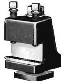
The Open Side Tool Post, sometimes called "European Tool Post" is convenient for working close to the face plate or chuck. Made of malleable iron and equipped with clamping bolt, two heat treated dog point screws, and drop forged rocker.
