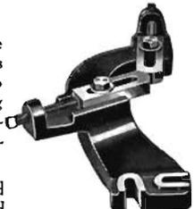
Slots in bottom of follower rest are used for attaching follower rest to carriage, and permit attaching or removing quickly, as it is not necessary to remove the screws from the saddle.
