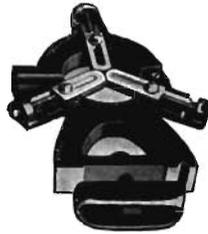
The jaws are made of cast iron, and if properly lubricated, will wear very little. The jaws are machined all over and have adjusting screws and lock screws for setting them in the desired position.
