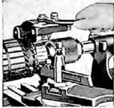
Truing an Armature Commutator and Undercutting Mica in the Lathe
