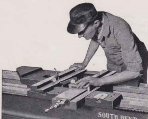
Testing the Cross Slide of the Saddle
