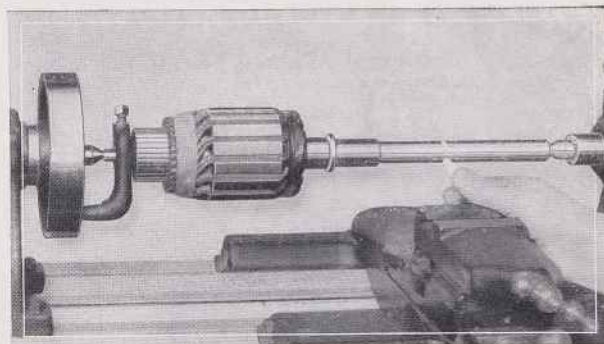
Testing a Bent Armature Shaft Between Centers on a 9-inch Lathe
