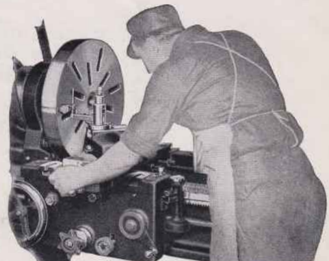
Testing Large Face Plate with Dial Indicator
