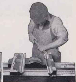
Scraping Saddle to Lathe Bed
