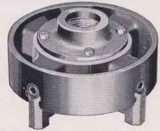
Chuck Fitted to Lathe Complete
