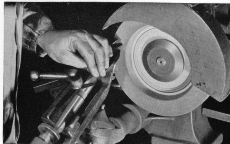
Sharpening a large drill on a pedestal type of drill grinder
