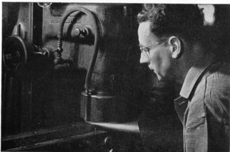
Vertical spindle type of surface grinder using a cup wheel
