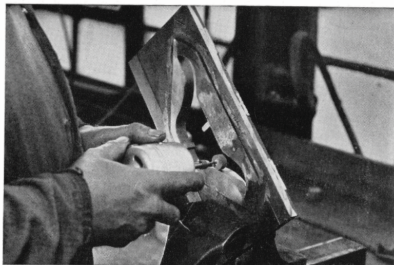
Portable high speed grinder with mounted wheel for die grinding
