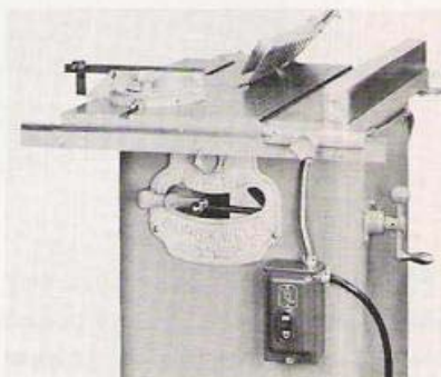
Arbor Tilted for 45° Bevel Cut
