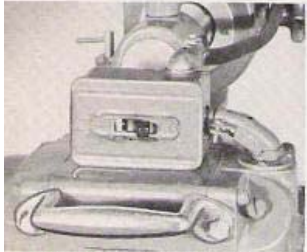
Motor control switch is at your finger tip, right at the motor unit pull handle. You can turn motor on or off without taking your eye off your work, or your hand off the handle.
