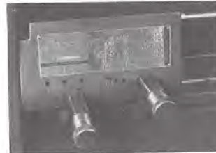
Converts a Logan plain change gear Lathe for quick change gear operation
