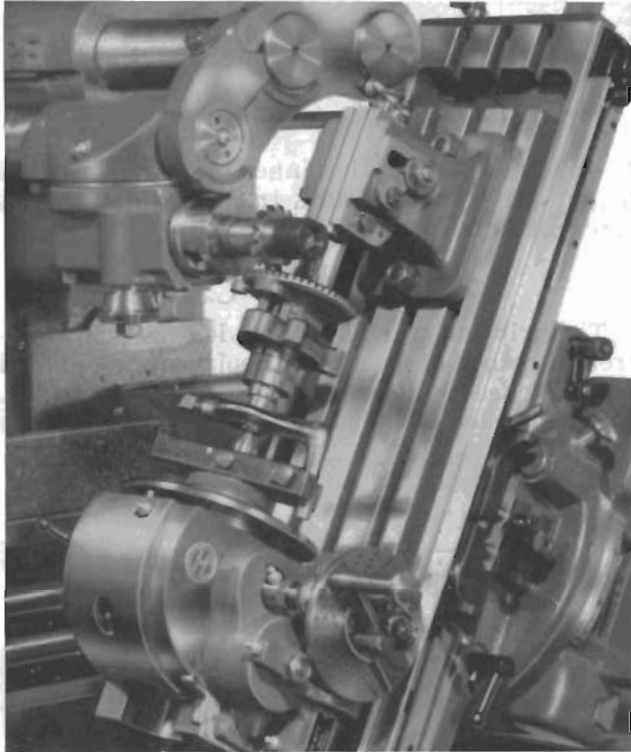
Fig. 18 (left). Milling teeth in bevel gear blank rigidly supported between centers. The work is mounted parallel to the table, and the table is set at zero and clamped, thus bringing the work in a plane parallel to the path of knee slide travel. The knee is then set to the desired cutting angle and fed horizontally to cut the teeth.
