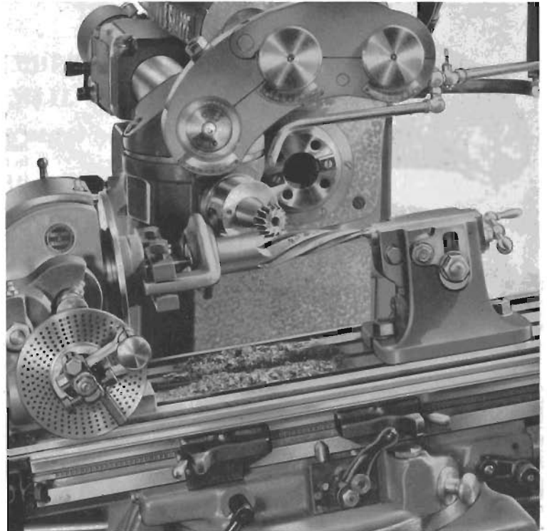
Fig. 22 (below). Milling slots in inserted-tooth cutter body. The work is mounted on an arbor and held securely between the centers of the universal spiral index centers. The table is set to 12° to give angle of this amount between sides of slot and axis. Knee is set to give 5° angle between bottom of slot and axis. Horizontal feed of the knee is used, with table clamped.
