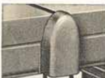
A guard encloses belt and pulley for maximum safety. These are the only moving parts, aside from the cutter head.
