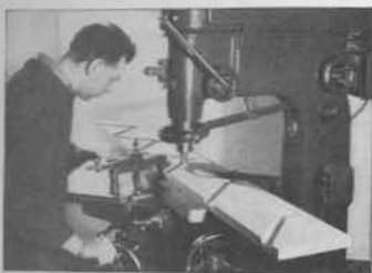
Cutting housings for string boards. Fixture in use dispenses with the need for marking out.
