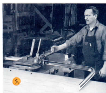
Forming tube with DI-ACRO HYDRA-POWER BENDER NO. 6.
