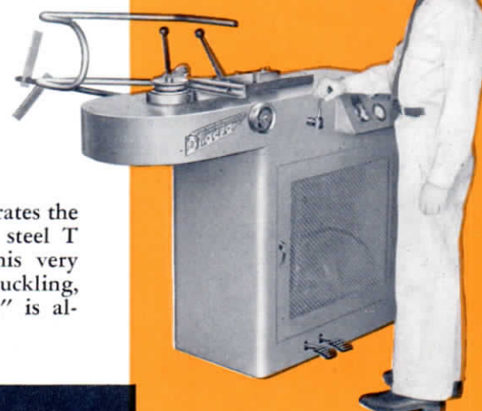
Forming tube with DI-ACRO HYDRA-POWER BENDER NO. 6.
