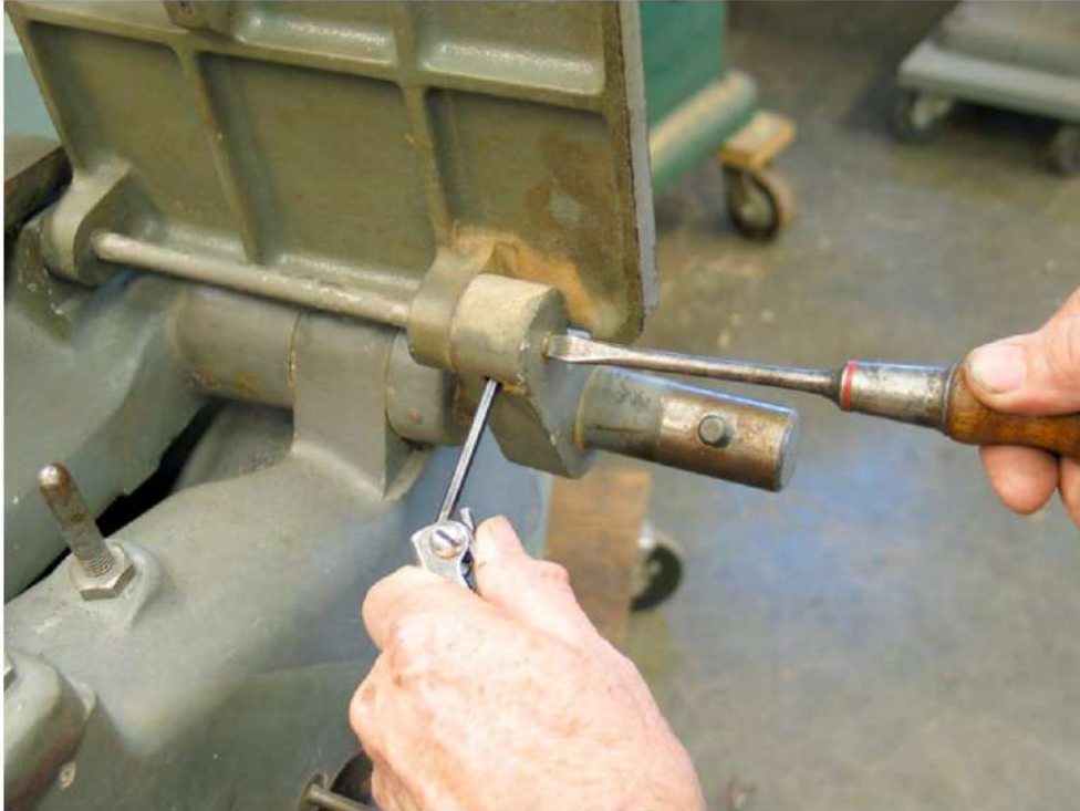
Figure 346 The position of the back table can be adjusted by loosening the rod setscrew and turning the slotted end of the rod with a screwdriver.
