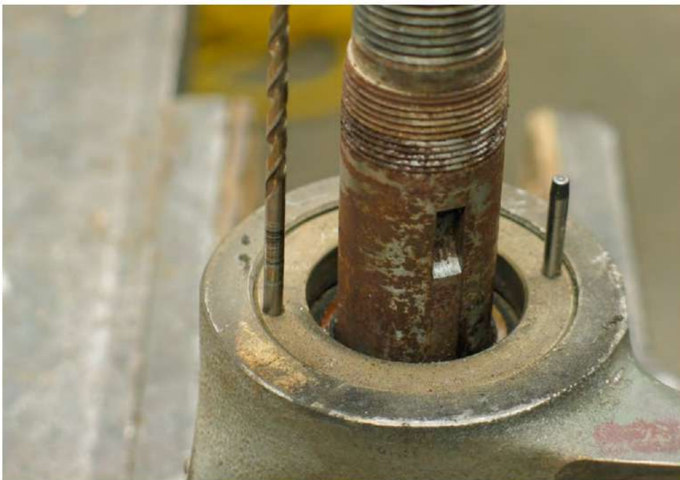
Figure 13 Under the pulley is another spanner ring holding the position of the outer race of the bearing. There is one of these rings on each side of the arbor housing. The arbor will have to be pressed out, putting pressure on the pulley end (shown here)
