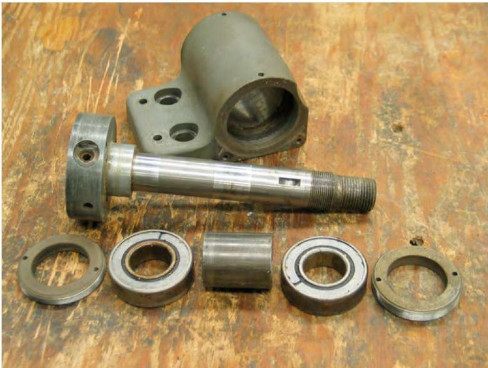
Figure 15 The entire assembly is shown here. When re-assembling, the two brass spanner nuts will screw in and out to adjust the position of the blade flange. There should be light hand pressure compression on these two nuts. That's all the preload needed.
