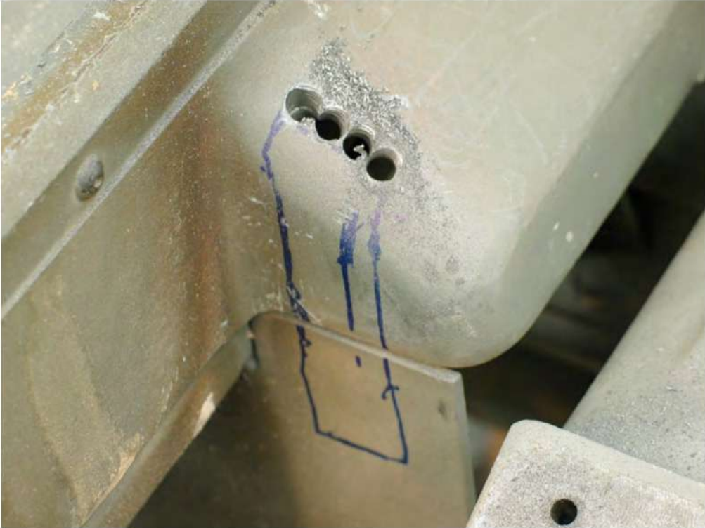
Figure 256 Holes neatly done. The sheet metal under the cast area will be cut away and not U-slotted as drawn.
