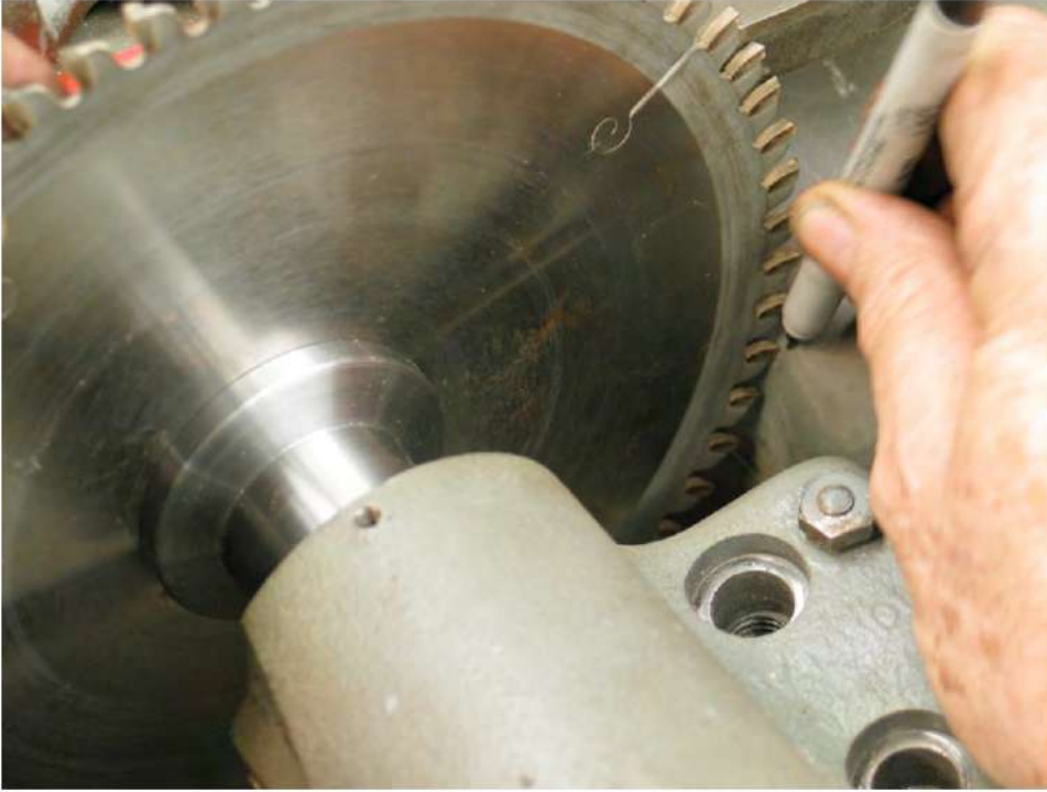
Figure 3222 With the 8-1/5" blade in the upper position, observe where the cuts need to be made and mark plenty of clearance with a marker. Keep in mind that the blade has to move laterally to come off the shaft.
