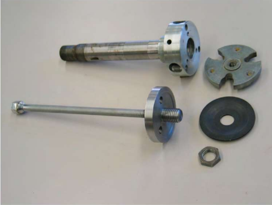
Figure 26 This is the new threaded faceplate showing the Unisaw nut and the Unisaw blade flange. Using the original arbor limits blade height above the table.
