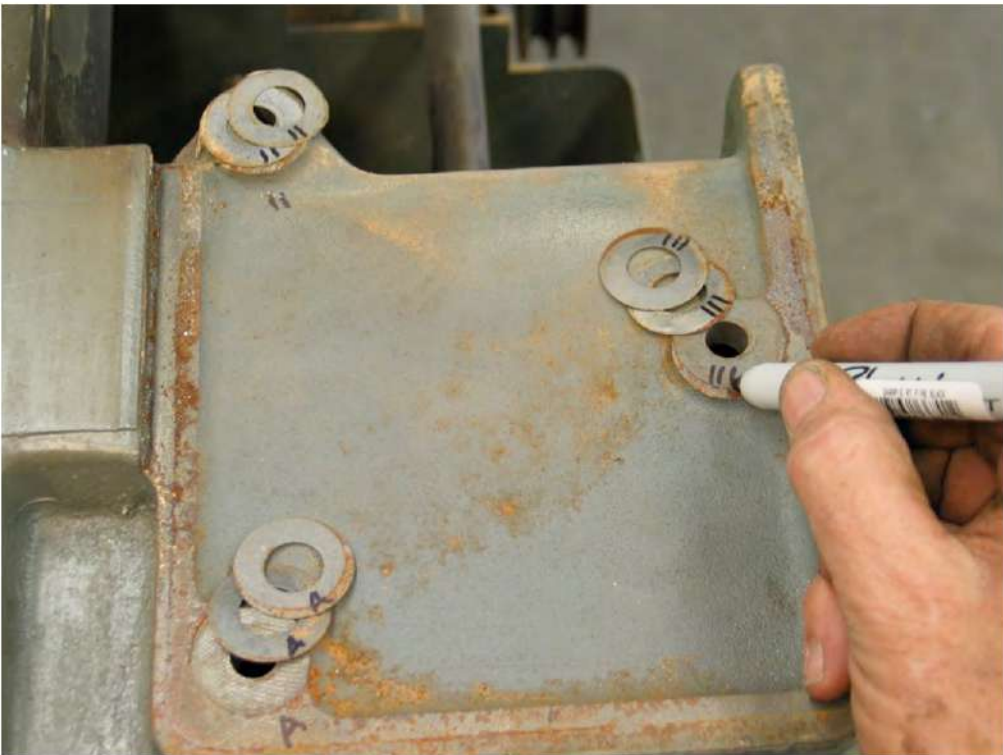
Figure 19 Mark well where the factory shims go.
