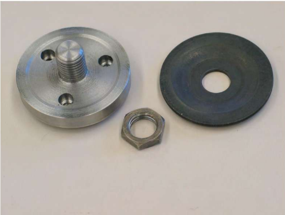
Figure 27 Front side of new faceplate. Note the countersunk holes for the cap screws. The machinist making this part will determine the dimensions.
