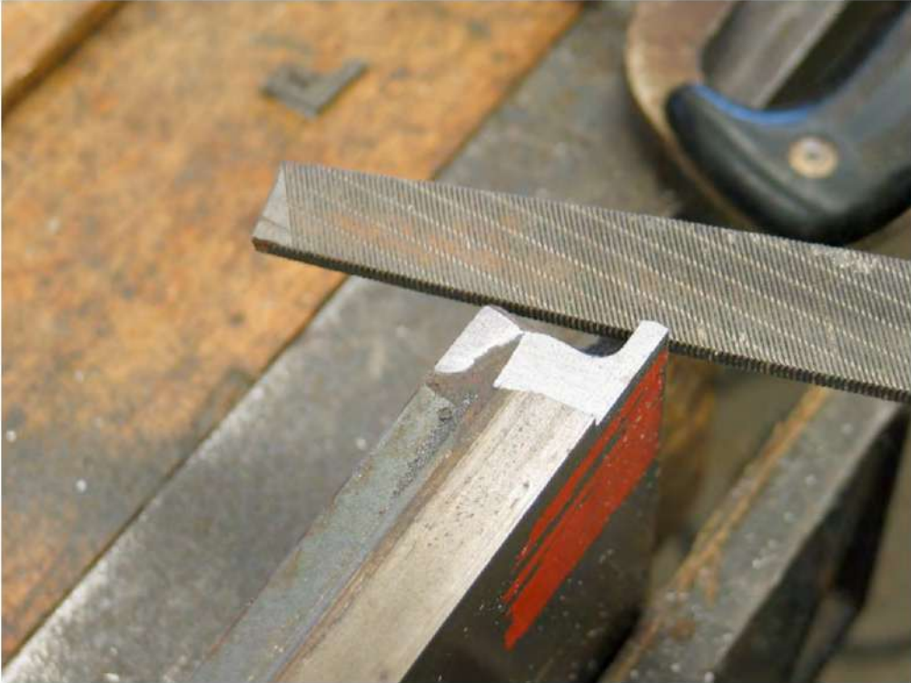
Figure 22 Clean up the hacksaw marks with a file.
