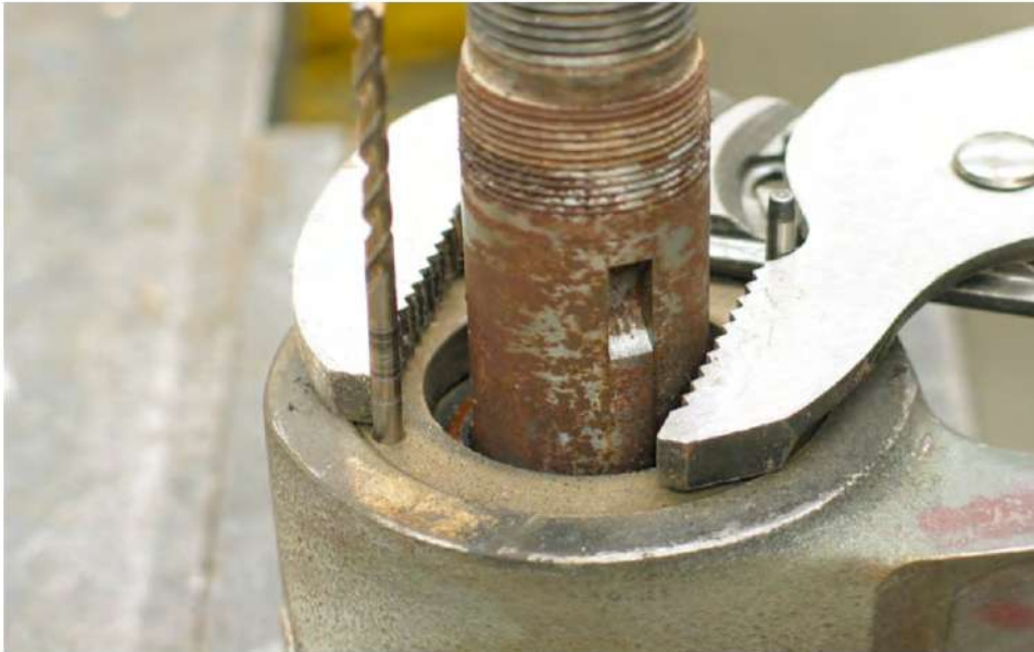
Figure 14 Only light pressure should be required to get the outer race spanner nuts turning as they put very little force against the bearings.
