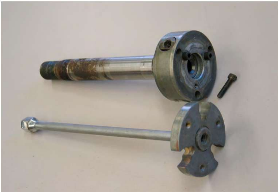
Figure 25 This is the original faceplate with drawbar and original shaft. The faceplate method uses the original shaft so a new one doesn't have to be made. The new faceplate will fit into the recess and be held in by the drawbar and the three perimeter 10-32 socket head cap screws.
