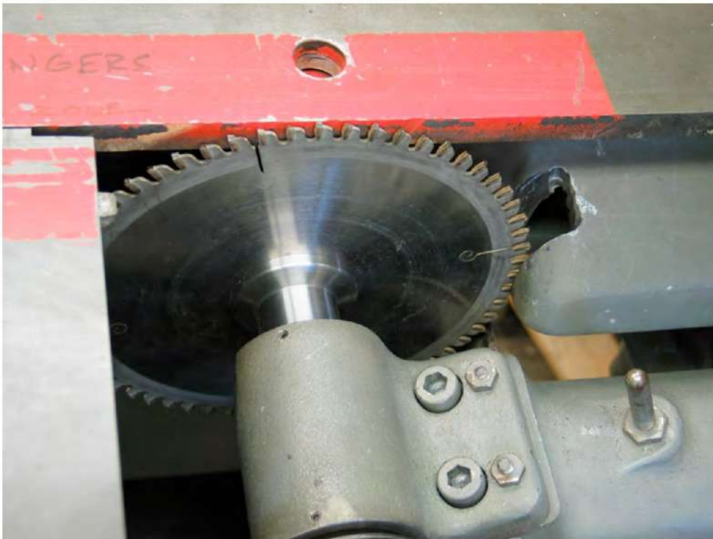
Figure 357 The installed blade ready to go.
