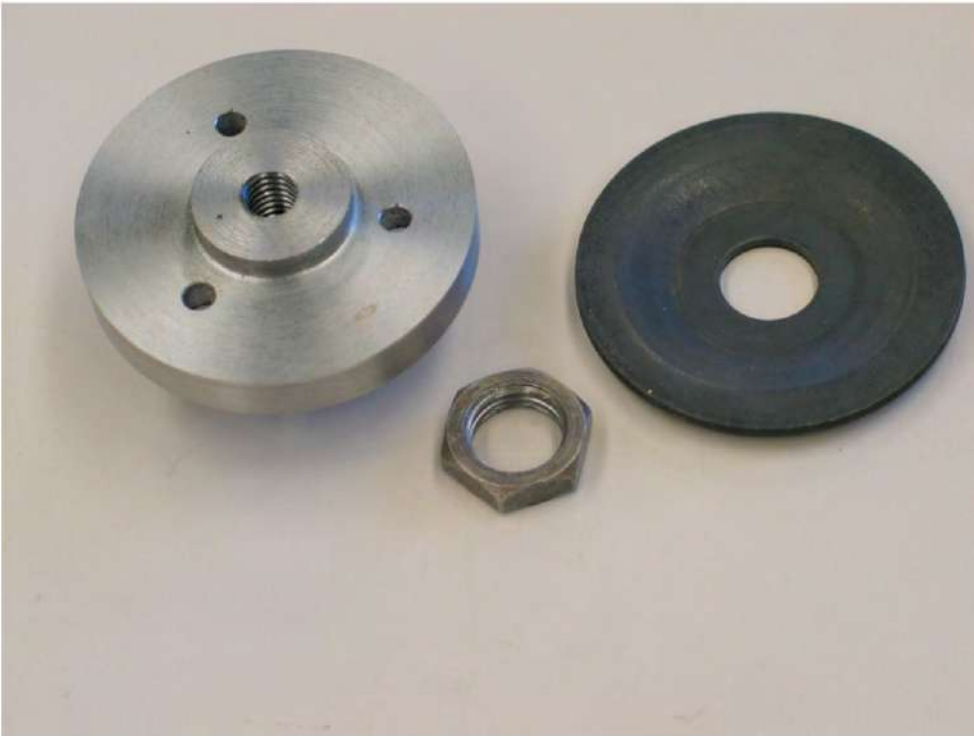
Figure 28 The back side of the faceplate showing threaded hole for 3/8-16 drawbar. This is an inexpensive fix, but not as accurate as an entirely new shaft.
