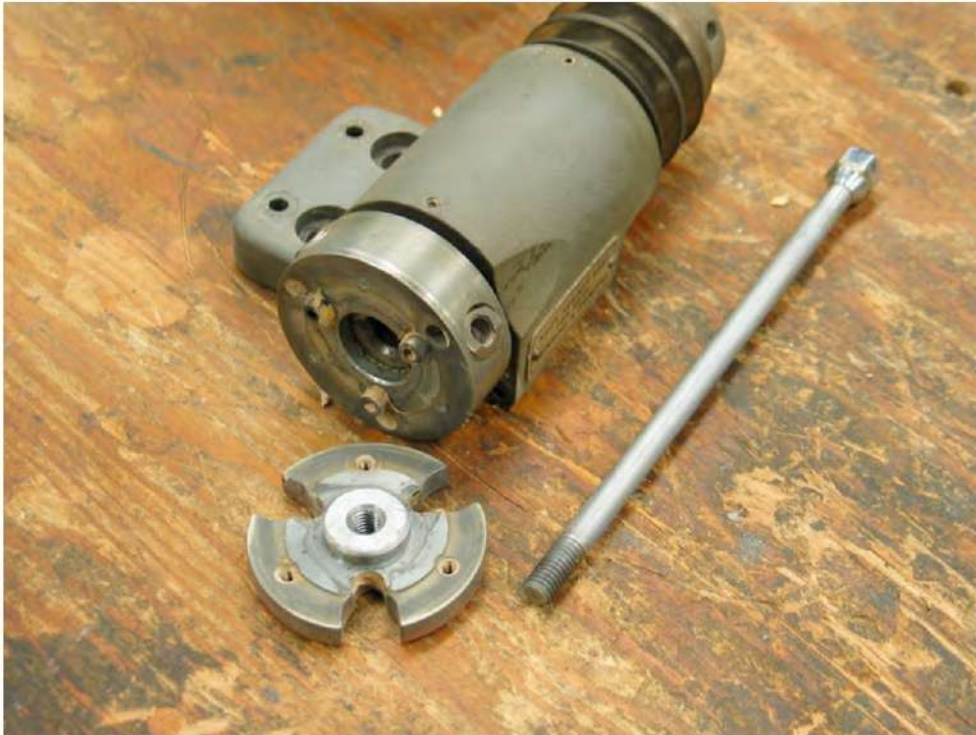
Figure 6 Drawbolt has been removed along with the face piece.
