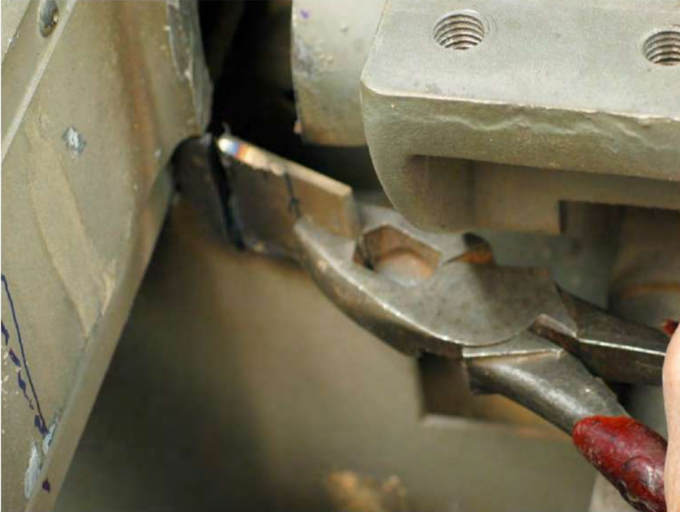
Figure 302 Once the two cuts have been made, pliers will worry out the waste.
