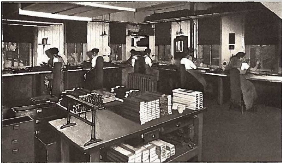
Section Inspecting Department, showing how every UNIVERSAL HACK SAW is inspected before packing, to prevent shipment of imperfect blades.
