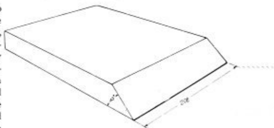
Showing a miter joint on wide stock
