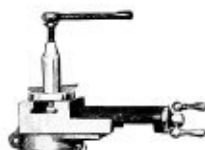
Compound Swivel Cross Slide and Tool Post easily removed from the carriage to allow use of hand Tool Rest Holder
