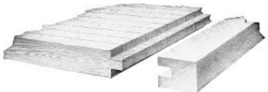
End Grain in tongue where bolster is glued at end of bench and then bolted
