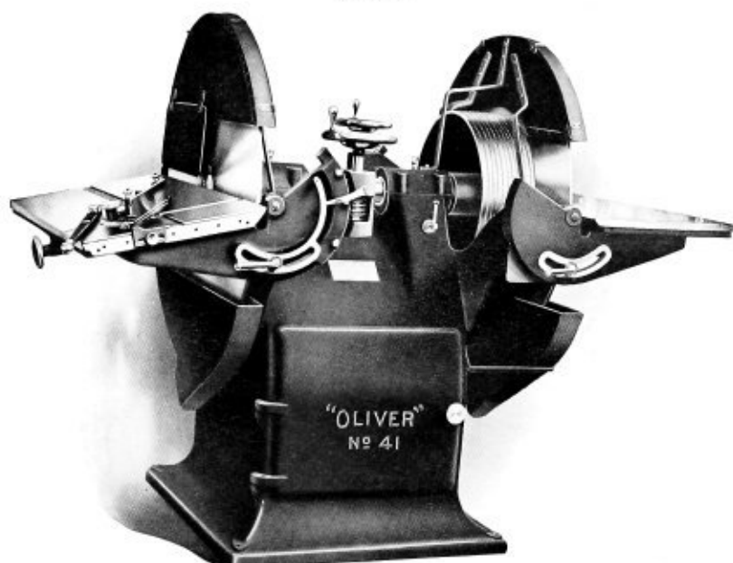
No. 41-B "OLIVER" DOUBLE DISK SANDER—37-inch Note the disk Guards and Dust Hoods Regularly Furnished
