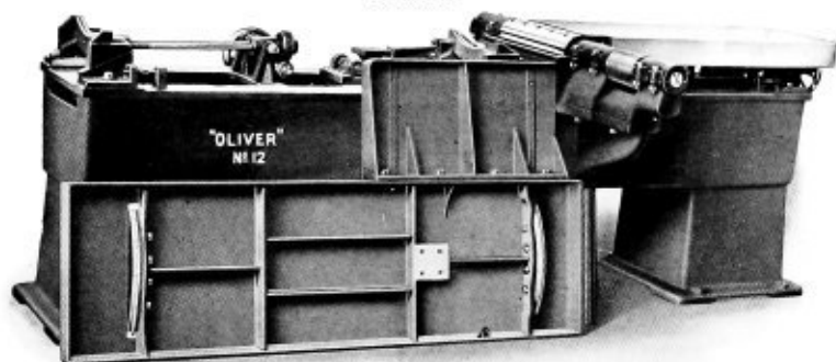
Rear View with operating table removed to show finished rockers and hand wheel worm and gear tilting device
