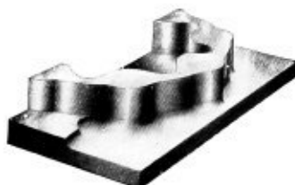
No. 1. The fillet and recess done by \frac{1}{2} " fillet cutter.
