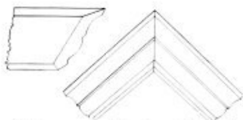
Showing compound angle and mitered frame molding
