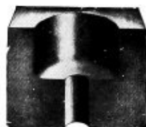
No. 5. Sample of work done with fillet cutter and 1" core box cutter. The large recess is 3\frac{1}{2} " in diameter.
