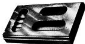
No. 6. Showing round and flat bottom mortises made with core and routing cutters respectively.
