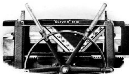
Showing the broad bearings back of bed and the gear and rack cover, etc.
