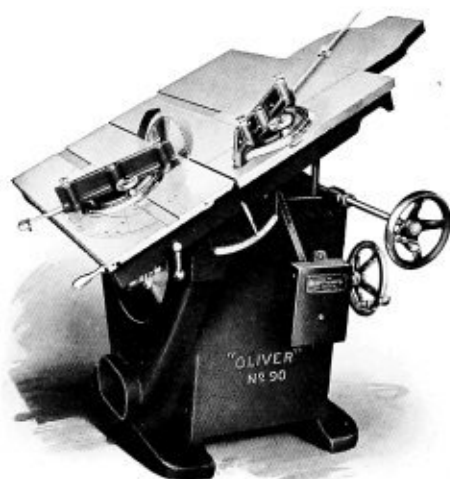
No. 90 "Oliver" Universal Saw Bench Showing Table Tilted to 30 degrees
