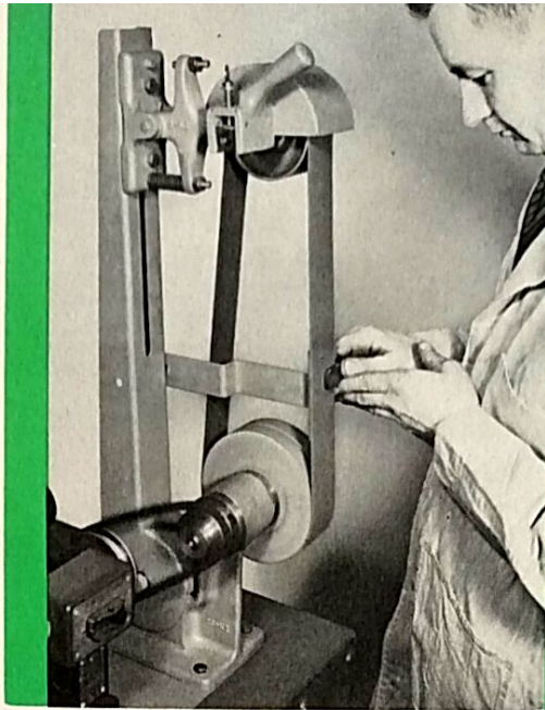
Using Platen on a CN-2 Handy Belt Grinder to clean up and square inside a fork-shaped piece. CN-2 Porter-Cable Handy Grinder.
