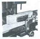
RIGID CHIPBREAKER assures smooth, clean, splinter-free cuts on #15 chain saw mortisers.
