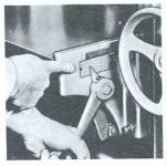
"Quik-Set" feature offers lever controlled table roll height adjustment from 0" to .040" (1.02mm) at a touch. Quik-Set eliminates friction and constant under-the-table roll adjustments.
