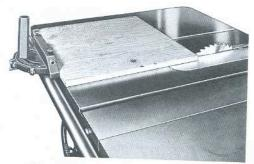
\*Extra Cut-Off Capacity table in front of blade is full 21" (533.40 mm) at 1" (25.40 mm) cut.
