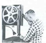
Counter-Balanced Guide Bar makes guide and blade adjustment safe and simple. Note telescoping guard completely enclosing blade above guide.
