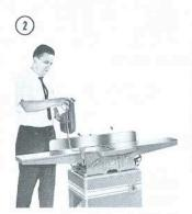
Exclusive Swing Away Guard remains attached to machine during rabbet operations.
