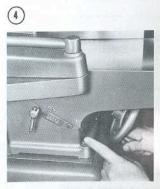
Quick, Sure Table Adjustments on precision dovetailed ways are easy to make, easy to read. Adjustable gibs compensate for wear, guarantee alignment. Lever-lock prevents table slippage during operation.
