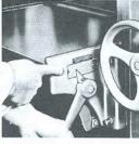
"Quik-Set" feature offers lever controlled table roll height adjustment from 0" to .040" (1.02 mm) at a touch. If you are tired of the "push-pull" planing method. Quik-Set eliminates friction and constant under-the-table roll adjustments.
