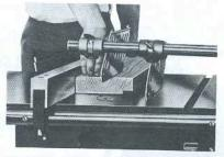
Maximum safety with rabbet or moulding cuts. Protection is provided by swinging guard leaves a see-through visor on top of guard.
