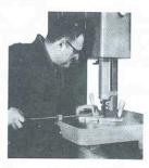
Screw Feed Attachment, fitted to table insert, offers maximum in feed control and safety for cutting smaller stock.
