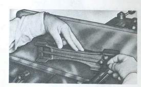
Anyone can set jointer knives or bed rollers speedily and precisely with this easy-to-use gauge. Variations are micrometer calibrated and are easy to read on this foolproof measuring instrument.
