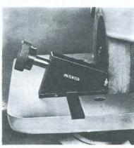
Sliding bracket is adjustable for different sizes of grinders and tool rests. Sides of grinding wheels may be dressed by moving bracket to fit side of tool rest. Bracket fits in "T"-slot of carbide tool grinder. Part No. 6028006. For 2200 Only.
