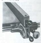
Fence Adjustment Fast and Sure from either side with Vernier control knob and top-reading front guide bar calibrations. Upper knob locks rear of fence. Fence is precision machined cast iron with tubular steel guide bars. Standard guide rails provide 25" (635.00 mm) cut to right of blade.
