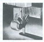
New upper and lower guide blocks with M-2 steel faced back-up bearings are standard with the Model 87. One set of 36" (9.52mm) inserts only is supplied as original equipment.
