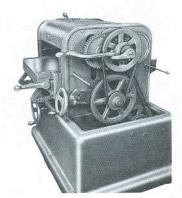
Belted Feed Drive Assembly is simple and trouble free. A combination of variable speed pulleys, V-belts, and heavy pitch gears provide smooth dependable feed rates without use of expensive and troublesome transmissions and gear-boxes.
