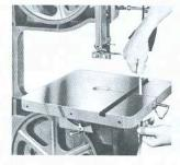
Side Takeout Slot for bandsaw blade eliminates necessity of split or narrow trunnions. Tapered pin keeps table surface flat.
