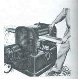
Feed Speed Adjustable from 15 FPM to 37 FPM (76.20mm/s to 187.96 mm/s) with variable speed pulley. Sets quickly for every stock or finish requirement.
