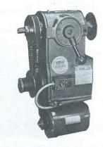
The Model 90 Lathe Drive System is a double reduction drive from the motor, through a jackshaft, to the headstock spindle. Isolation of the motor mount and the use of a jackshaft combine to minimize vibration.
