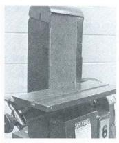
Removable tilting table (15° up 45° down) can be used with either disc or belt.
