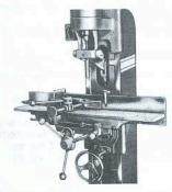
UNIVERSAL TABLE - assures complete flexibility for mortise cuts at any angle. Fast, simple 45° right or left tilting, 14'' (355.60) vertical and 12'' (304.80) longitudinal table adjustment.
