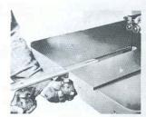
Table Insert Quickly Removed for fast blade change. Note deep flange on precision-machined table for extreme rigidity.
