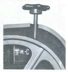
Eye level blade tension scale shows correct tension for different blade widths. Adjustable from front of machine.
