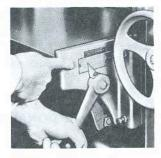
"Quick-Set" feature offers lever controlled table roll height adjustment from 0" to .040" (1.02 mm) at a touch. Quik-Set eliminates friction and constant under-the-table roll adjustments.
