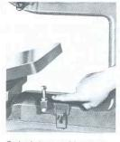
Swivel type table stop. Positive table stop at 90° or is easily moved for a 15°
