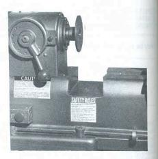
Choice of Straight or Gap Bed. 12" (304.80mm) stock capacity over straight bed, 17" (431.80mm) stock capacity over gap.
