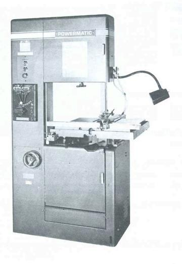
In addition to the rigidity and extra strength standard with Powermatic® bandsaws, the new "dynamatic" has improved on this feature with a new unitized steel frame. Deflection of the upper housing under full load is minimal.
