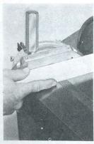
Optional miter attachment for straight and angular sanding.
