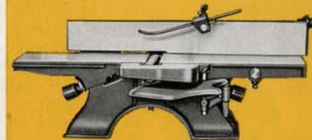
While rabbeting, or adjusting the knives, the safety guard is simply slipped under the overhanging arm.
