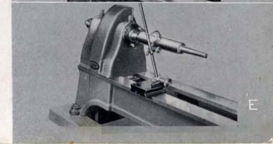
Photo E—Frequent tests are made during manufacture to assure utmost precision. Here a delicate gauge is used to check accuracy of the spindle. This will be recognized as a severe test, the reading being taken at a distance from the spindle. In this position any error is magnified. Following this test the tail stock (with center removed) is slid up to this test bar to check alignment of the tail stock with the head stock.
