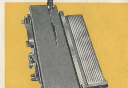
View from above showing how splitter spreads saw cut slightly. This greatly facilitates sawing.
