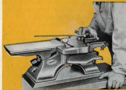
The cutter head is tested for alignment with the table by a delicate gauge which shows variations in
