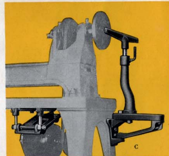
Photo A—Showing the "900" lathe mounted on the 9LB15 bench. This set up is for woodworking. Metal working requires the use of a jack shaft mounted on the lower shelf with the motor suspended below.
