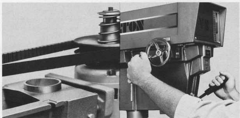
Variable Speed Drive
